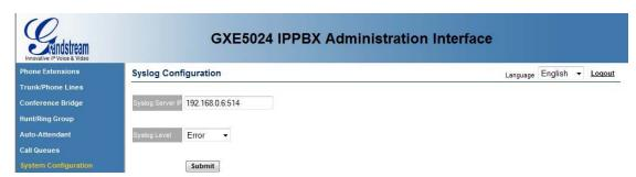
Enter the IP address of the Syslog server in the *Syslog Server IP* field, and use the *Syslog Level* drop-down box to specify the level. When done, click the **Submit** button to save the changes.
